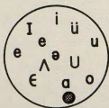
(c) VOWEL-CIRCLE DISPLAY, SHOWING "DOT" (CROSS HATCHED) FOR SPOKEN "A" AS IN "FATHER".
