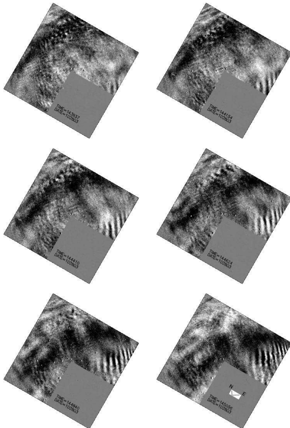
Figure 4. A sequence of time difference images taken by the Aerospace near-infrared camera between \sim 1440 and 1450 UT. The time difference image is the difference between two subsequent raw images which were taken every 1 min. The time and date are shown in the SE quadrant. The images have been flipped and rotated such that they have the same orientation as that in Figure 2 with north at the top and east to the right. Each image has a size of 256 \times 256 pixels. The central 128 pixels correspond to \sim 61 km.
