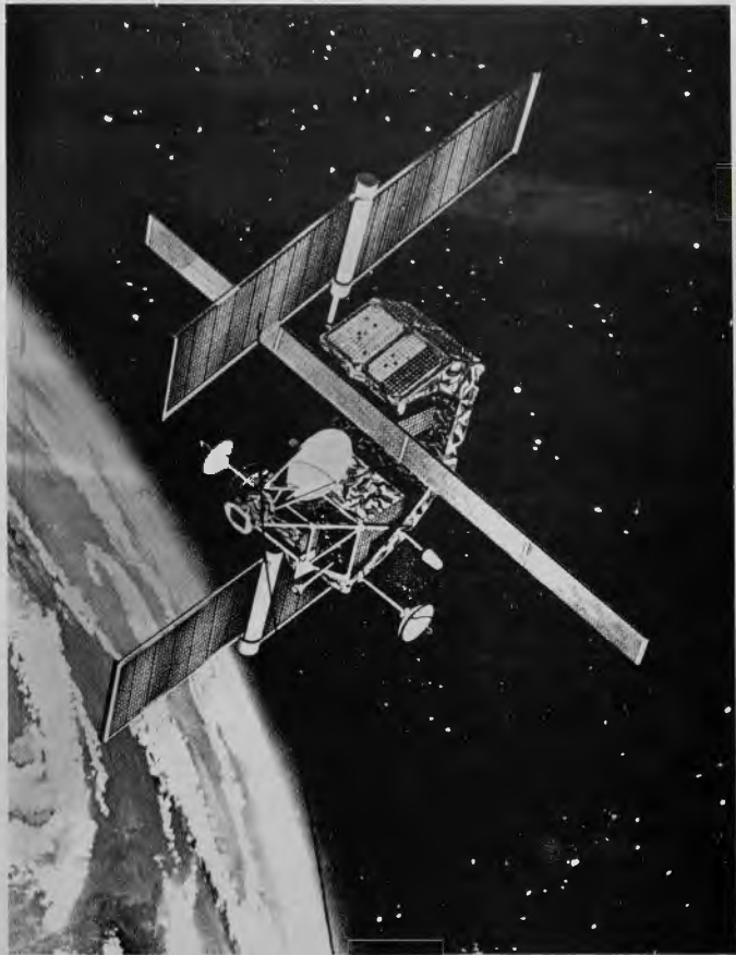
Fig. 12 Retrievable carrier concept based on Spacelab half-pallet.
