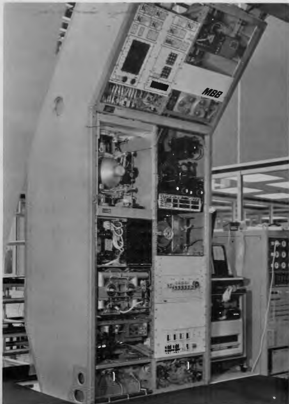
Fig. 4 Material sciences double rack facility for FSLP.
