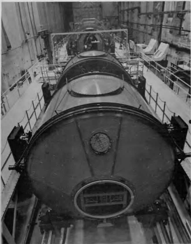
Fig. 3 OSTIA-1 payload and Spacelab engineering module being integrated into the Orbiter cargo bay.
