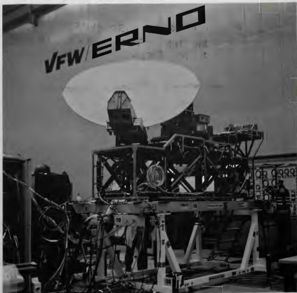
Fig. 5 FSLP experiments integrated into payload—on the European bridge assembly.
