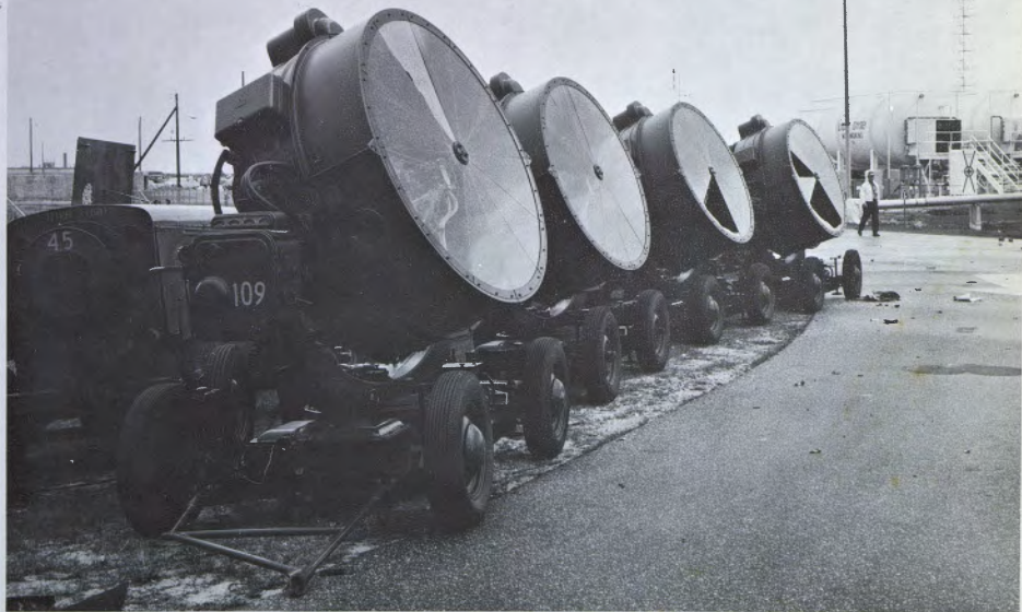
Fig. 4 SEARCHLIGHTS DAMAGED BY SHOCKWAVE
