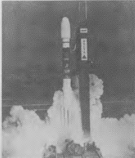
Figure 10. New 10-ft Fairing is Now Available as an Option—Shown on Delta ROSAT Mission for NASA on 1 June 1990
