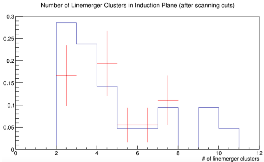
FIGURE 5.22: The number of Linemerge clusters in the Induction wire plane for data (red) and MC (blue) after the scanning cuts. Both have been normalized to one. Figure from [1].
