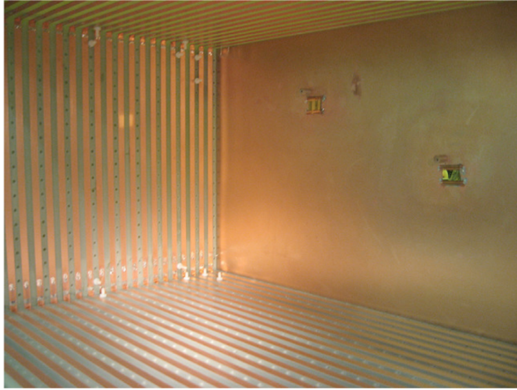
FIGURE 3.4: Inside the ArgoNeuT TPC. The copper strips lining the TPC is shown, attached to the G10 TPC frame. The solid copper sheet shown is the cathode plane. Figure from [15]
