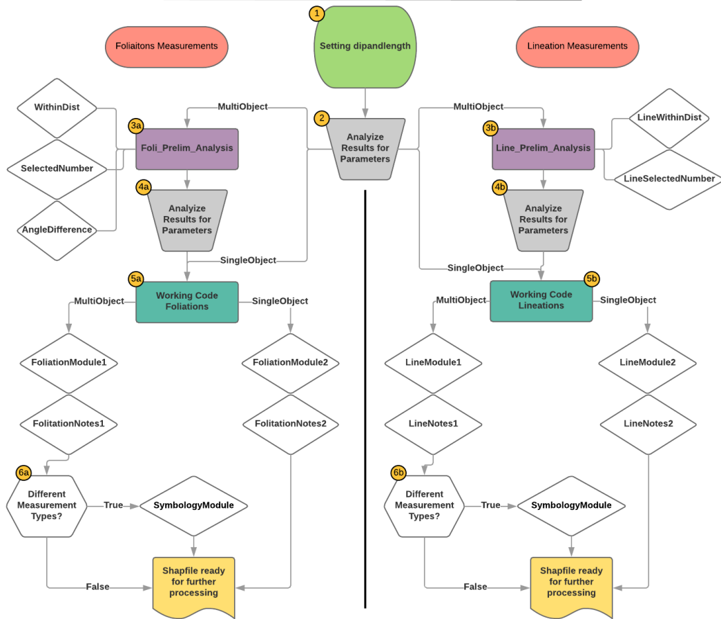
Figure 12 Shows the overview of the arcpy workflow created in this project, including all the lead-scripts and modules used in each of the four different workflow paths. 1. First the Settingdipandlength lead script code is used on all datasets simultaneously to create the populated Length and empty Dip fields. 2. The Length field can be analyzed to determine parameters required for the future scripts, such as the LenMin and LenMax, as well as any constraints on vertical measurements. Before moving onto step 3, the user will have to determine which of the four workflows the data matches, either foliation or lineation, and multi-object or single-object. However, the single-object paths skip steps 3 and 4. For multi-part objects, steps 3a & 3b , for foliations and lineations respectively, involve using the preliminary analysis lead scripts, that run either three or two modules on each dataset or shapefile being worked on at a time. In 3a, the Foli_Prelim_Analysis runs the WithinDist, SelectedNumber and AngleDifference modules on multi-object foliation datasets. In 3b, the Line_Prelim_Analysis runs the LineWithinDist and LineSelectedNumber, the lineation equivalents of the WithinDist and SelectedNumber foliation modules on multi-object lineation datasets. 4a. & 4b. These modules themselves create fields, one for each module, with values that must be used to populate the parameters of the Working Code lead scripts in step 5. Thus, in step 4 of either of the foliations or lineations workflows, the user must determine the necessary parameter values from the results of the preliminary analysis and input them into the correct working code script. 5a. & 5b. Depending on whether the current dataset contains multi-object or single-object measurements, the user will specify the either the number 1 or number 2 modules respectively in the working code lead script. Then once the modules and necessary parameters are selected and entered, the lead script can be run, producing the final azimuth measurement data. 6a. & 6b. Depending on whether there are multiple types of structural geological measurements in the dataset will determine whether or not the SymbologyModule should be used or not. If not, the symbiology values should be manually entered during post script processing.
