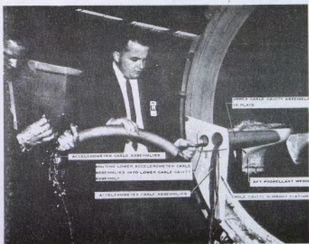
Figure 7. Installation of Accelerometer Cables in Cavity Assemblies
