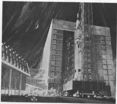
Figure 13. Close-up view of the Vertical Assembly Building and Saturn V on crawler-transporter.
