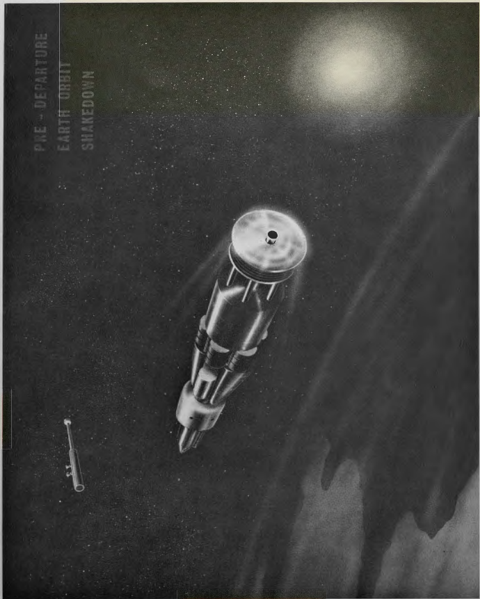
Fig. 11—Fully loaded nuclear pulse vehicle in earth orbit shakedown cruise prior to departure
