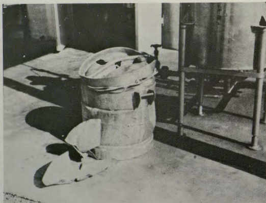
FIGURE 2. HYDROGEN PEROXIDE DRUM THAT EXPLODED IN STORAGE
