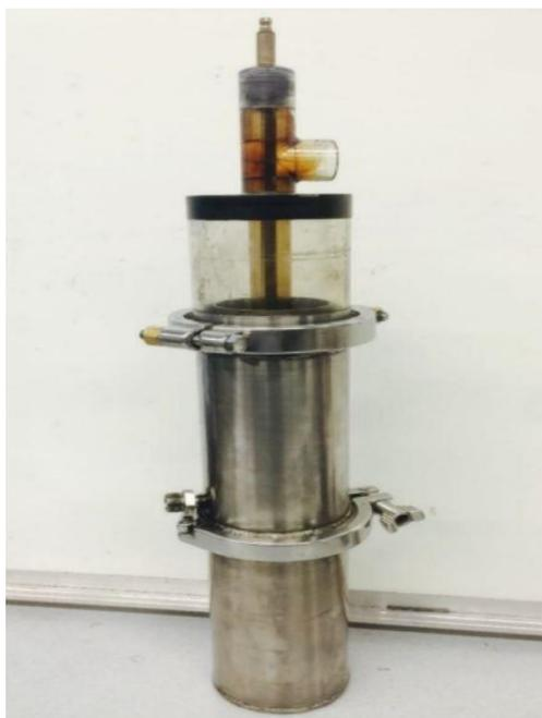
Figure 4.6 Electrostatic precipitator
