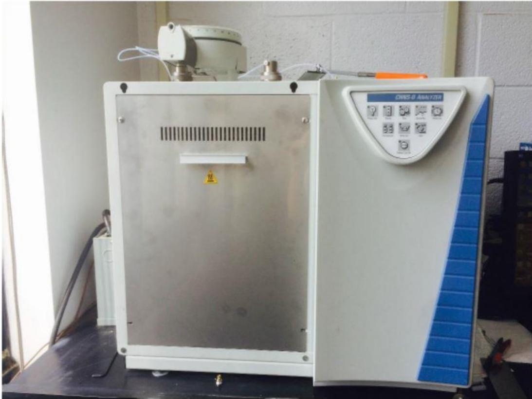
Figure A.1 Elemental analyzer for CHNO
