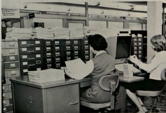
APPLICATION: MATERIEL RELEASE ORDER (MRO) HISTORY AT NEW CUMBERLAND ARMY DEPOT. AT THE LEFT, PRIOR TO CONVERSION TO MICROFILM, 438,000 EAM CARDS WERE STORED IN SEVEN CARD CABINETS AND LISTED ON COMPUTER PRINTOUT SEVEN FEET HIGH. THE SAME INFORMATION IS NOW AVAILABLE ON SEVEN 100 - FOOT REELS OF MICROFILM.
