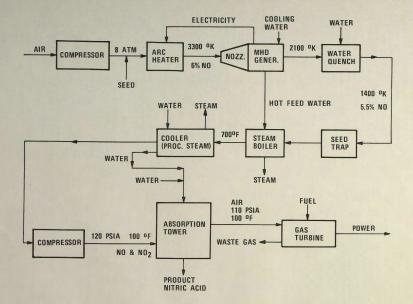
Figure 1. High Temperature Arc Nitrogen Fixation Process
