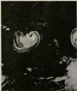
Figure 11. Threshold IR depiction. The data of Figure 10 has been separated into four temperature ranges with delineation at 250K, 230K, and 210K.
