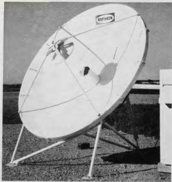
Figure 7. Thin Route Transportable Earth Station
