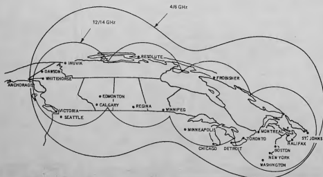
Figure 8. Dual Band Antenna Coverage for F4
