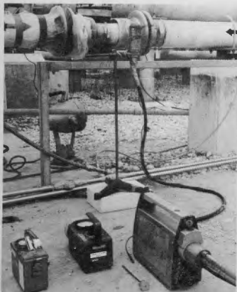
FIGURE 31 - FIELD RADIOGRAPHIC INSPECTION OF AN INVAR PIPE WELD IN VACUUM JACKETED PIPING
