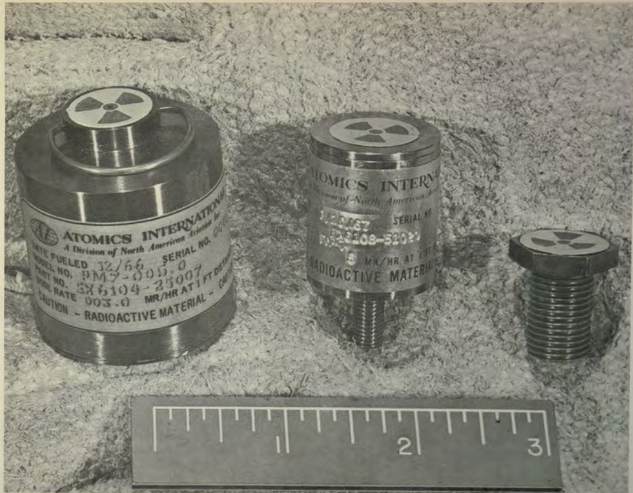
6. Typical ThermoPac Heaters
