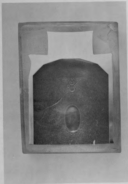
FIGURE 8. MACROPHOTOGRAPH OF A SECTION THROUGH AN INNER GIMBAL PREFORM SHOWING PRESSED INTERNAL DETAIL Specimen is shown in its metallographic mount.
