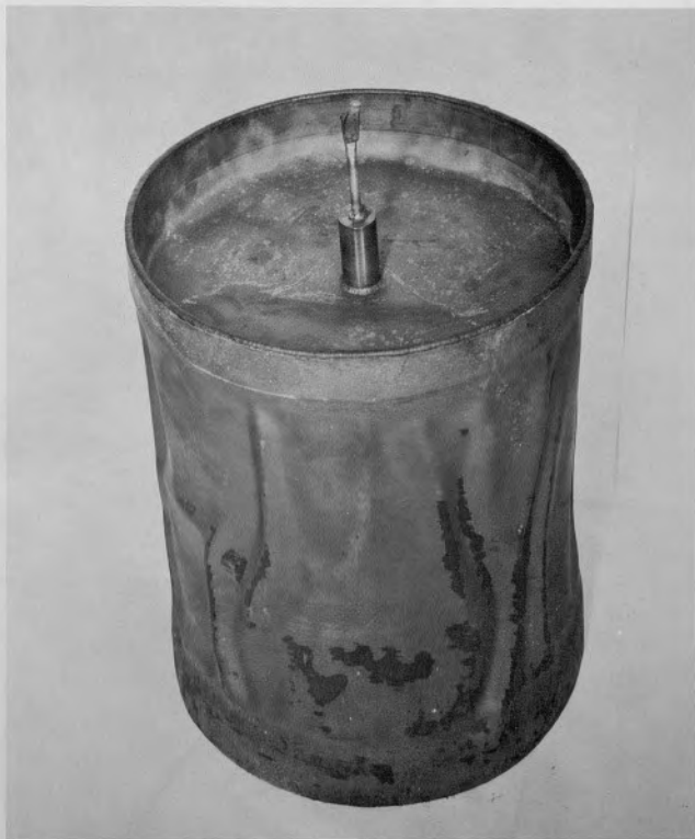
FIGURE 6. CYLINDRICAL CONTAINER USED FOR HOT ISOSTATICALLY PRESSED BERYLLIUM INNER GIMBAL
