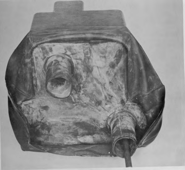
FIGURE 4. HYDROPRESSING SPECIMEN AFTER REMOVAL FROM THE STEEL BACKUP
