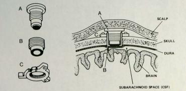
Figure 3. Intracranial Pressure Transducer/Transmitter Assembly. A) Transmitter B and C) Components of the Mounting Fixture
