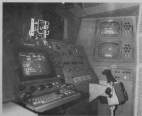
b OPERATOR COMPLEX INTERIOR CONFIGURED AS THE AFT FLIGHT DECK OF THE NASA SHUTTLE ORBITER
