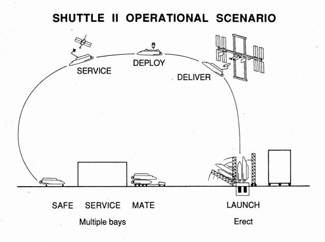
Figure 10.- General operational scenario for a Shuttle II vehicle.
