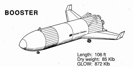
Figure 9.- Views of the Shuttle II orbiter and booster.
