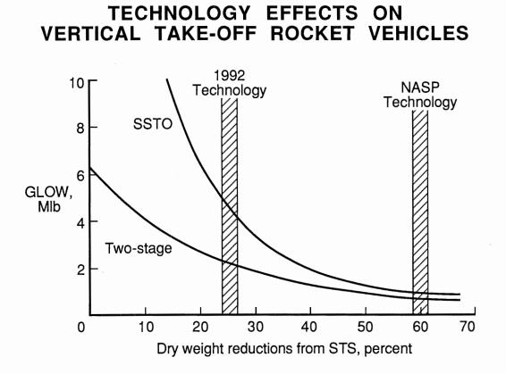
Figure 5.- Effects of technology advancements on gross lift-off weight (GLOW) of rocket vehicles.
