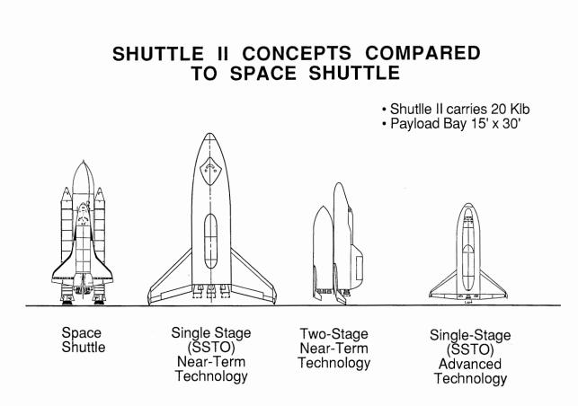
Figure 7.- Several Shuttle II design concepts compared to the Space Shuttle.
