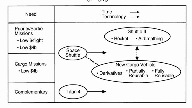
Figure 1.- Space transportation architecture options based on mission requirements.
