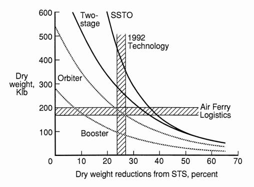
Figure 6.- Effects of technology advancements on dry weights of rocket vehicles.
