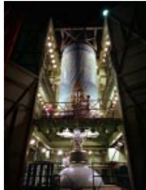
Figure 5: High fidelity prototype of the Single Engine Centaur undergoing structural testing in Lockheed Martin's Vertical Test Facility.
