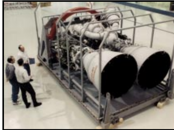
Figure 4a : Integration and assembly pathfinders have been performed with the high fidelity prototype RD-180, shown here in Lockheed Martin's Final Assembly Building (FAB)
