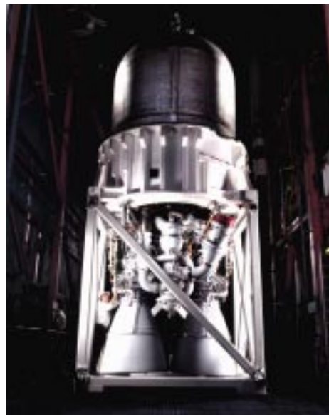
Figure 4a : Integration and assembly pathfinders have been performed with the high fidelity prototype RD-180, shown here in Lockheed Martin's Final Assembly Building (FAB)
