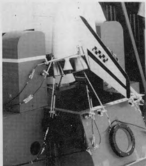
Figure 6 Duct Inlet Anemometers
