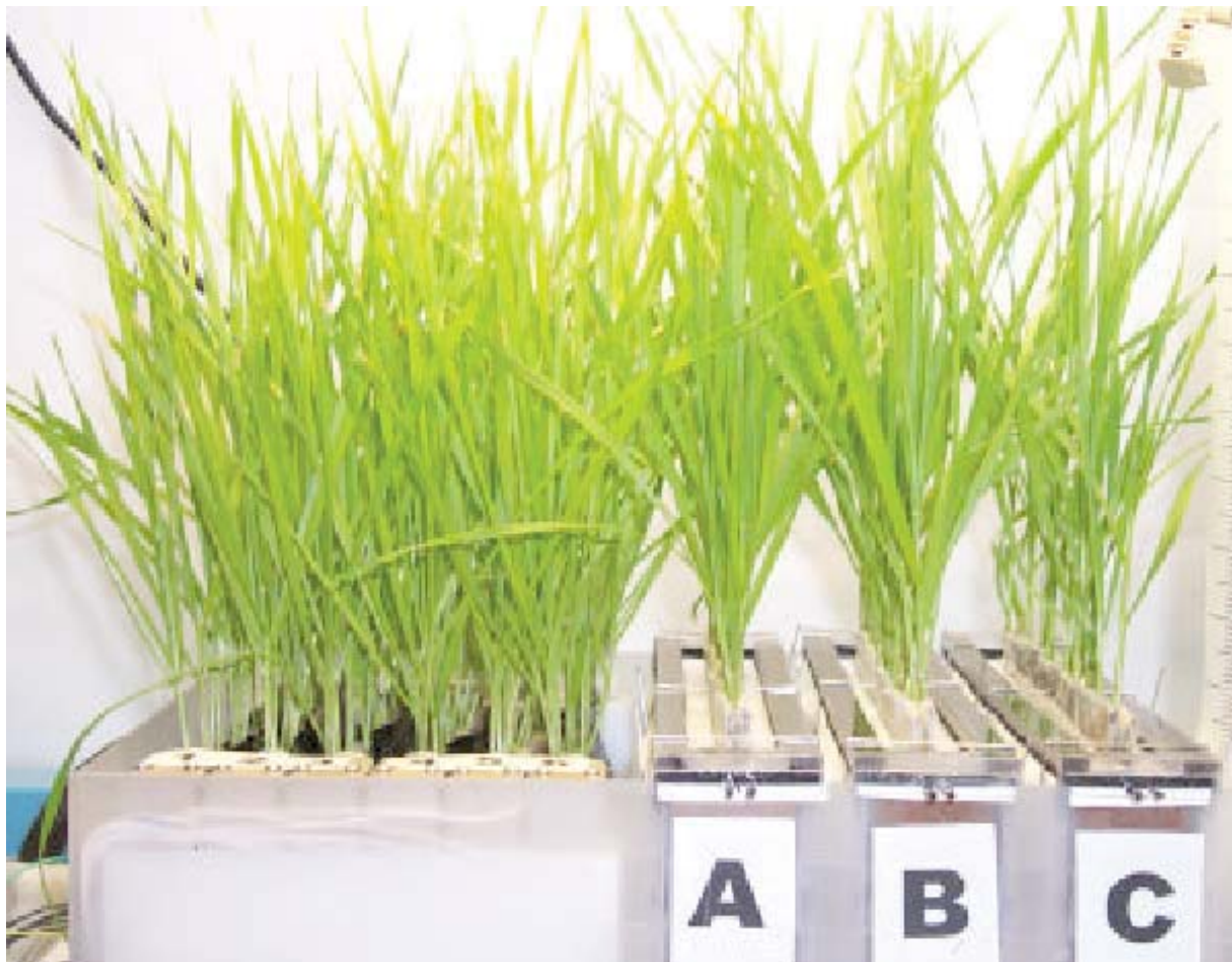
Figure 1. Porous Tube Insert Module (PTIM) Prototype Apparatus. The wheat plants depicted are the result of an 18 day ground experiment. The left half of the apparatus consists of six porous tubes nutrient delivery systems (PTNDS), and the right half consists of three substrate nutrient delivery systems (SNDS). Each PTNDS and SNDS unit is capable of being independently controlled with respect to water provision regime.
