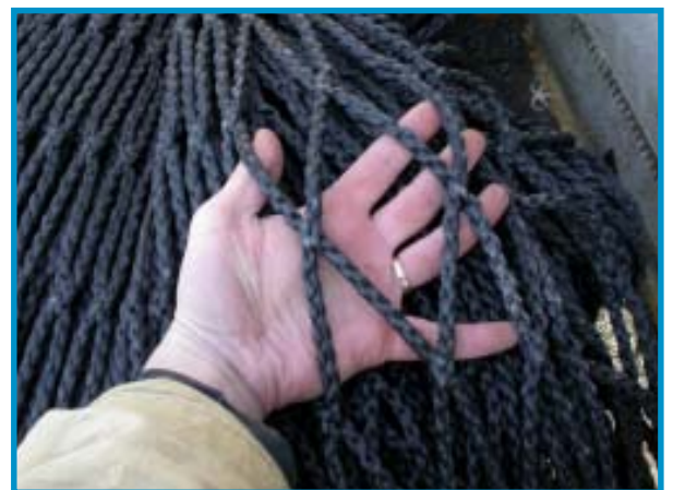
Figure 2. Knotless twine used in Experimental codend.
