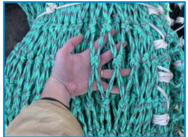
Figure 1. Knotted twine used in Control codend.
