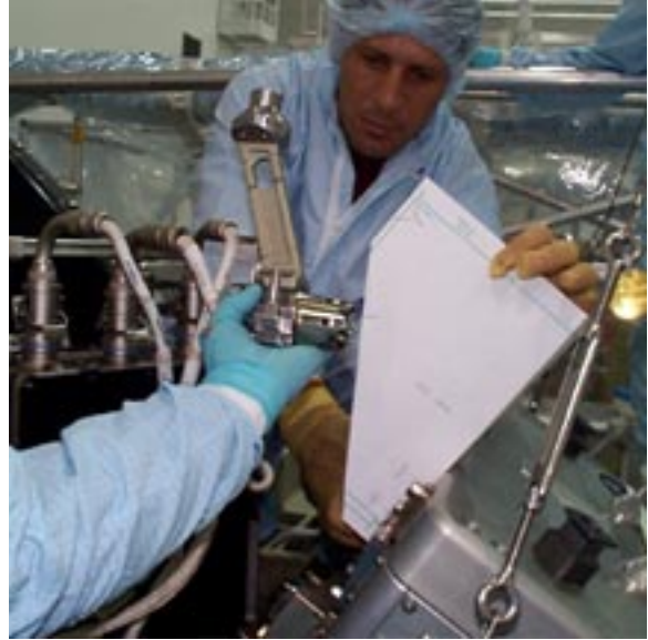
Photo #11 - Slings prevented STSD doors from being opened during dynamic fit check. Solution, create template of door.
