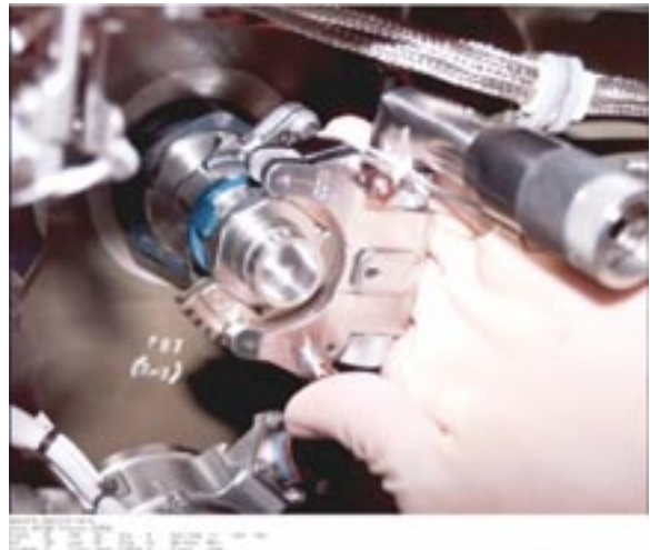
Photo #13 - Fluid fitting torque device used to assure surrounding hardware will not interfere with operat
