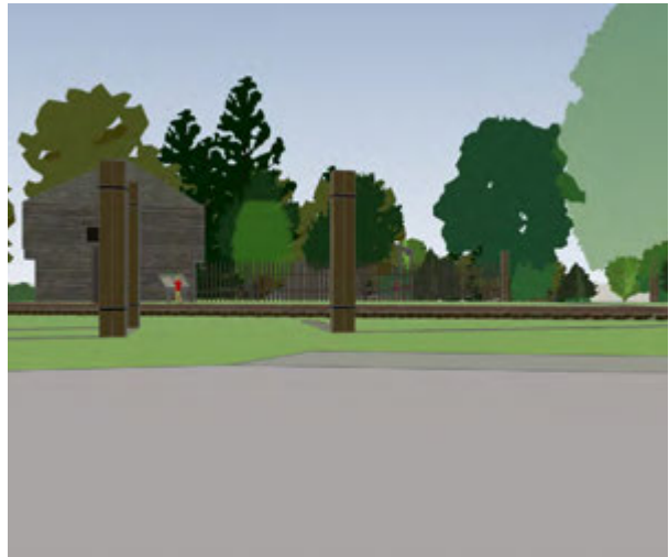
Model view showing the proposed 8' high stockade fence segments, 10' wood posts on corners of Fort buildings, and proposed tree planting to screen the pavilion.
