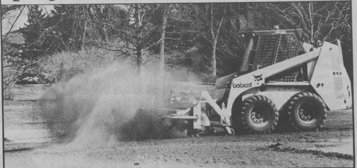
A sweeper-equipped Bobcat raises up clouds of grit from the pavement as it makes its rounds around campus. (Lachowski Photo.)
