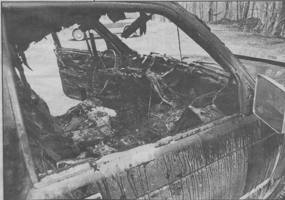
This 1985 Chevrolet S-10 Blazer belonging to Donna M. Olejniczak was destroyed by fire while parked at the Orono Post Office Wednesday morning. The Orono Fire Department theorized that the blaze began under the dashboard, but couldn't tell for sure from the wreckage. Nobody was hurt. (Page photo.)
