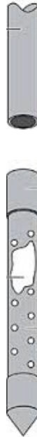
Figure 5. An example of a completed well made of PVC pipe, ready for installment in the meadow. Adapted from http://www.solinst.com/products/direct-push-equipment/615-drive-point-piezometers/datasheet/standpipe-piezometers.php
