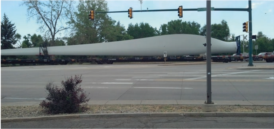
Fig. 5.2 Very large wind turbine being transported by train (Source: Michael E. Grass)
