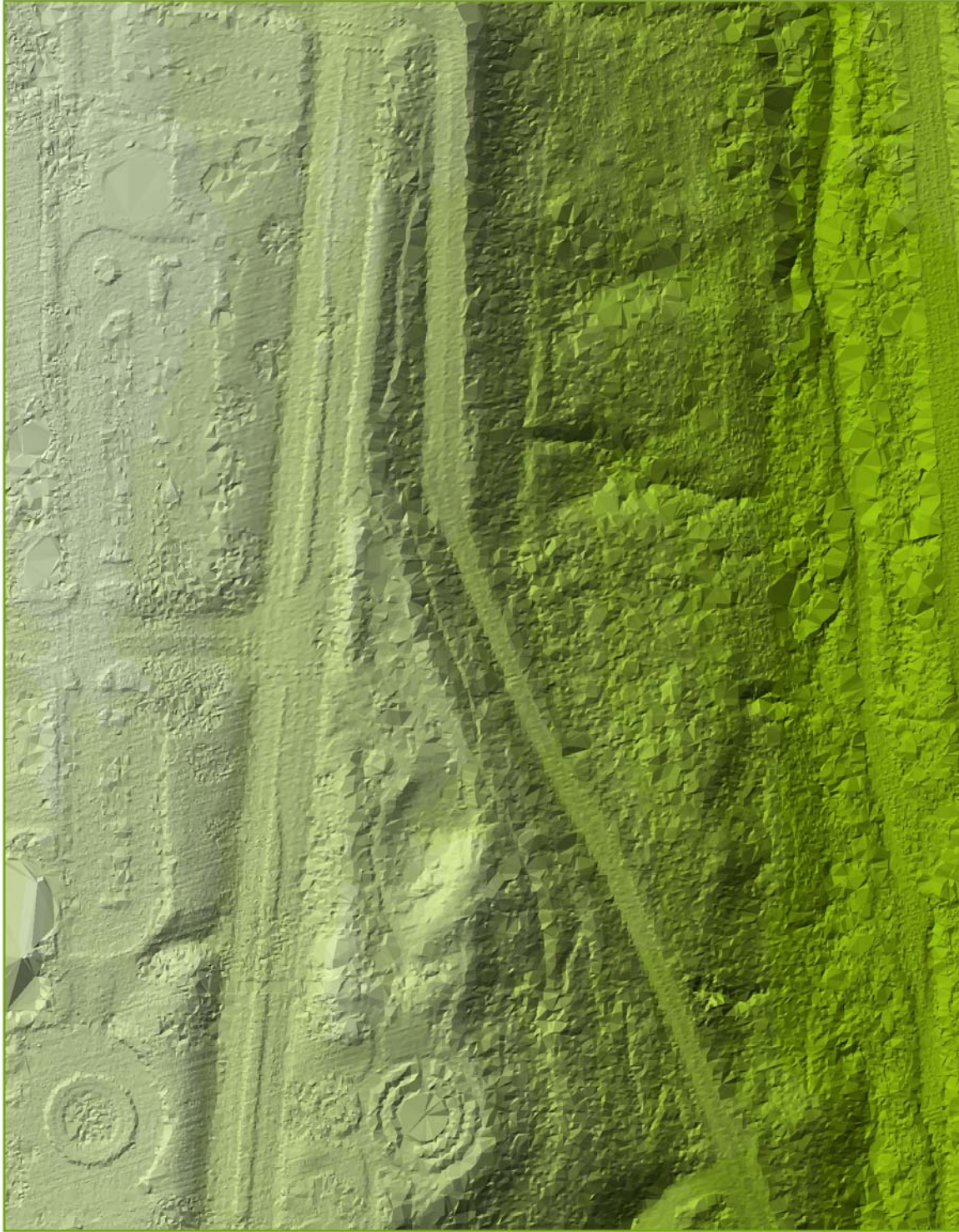
Figure 29. 3-D bare-earth surface map generated from lidar DEM.
