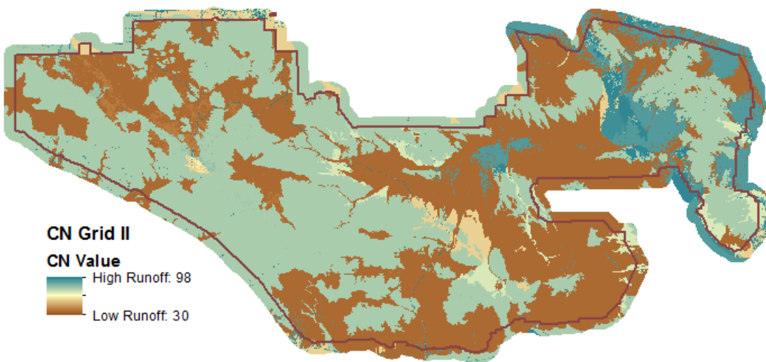
Figure 4.4: CN grid generated from ARC II values. This grid is one of three choices the user has when creating a runoff product
