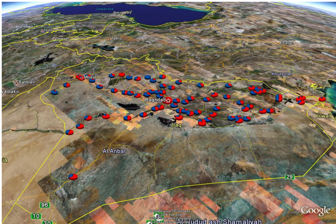
Figure 6. Example of Arc2Earth. Pie chart symbology was transferred from ArcMap to a KML file for viewing in Google Earth. Pie charts represent the percentage of the Iraqi population that is urban or rural in each district. (Source: Google, DigitalGlobe, Government of Iraq)
