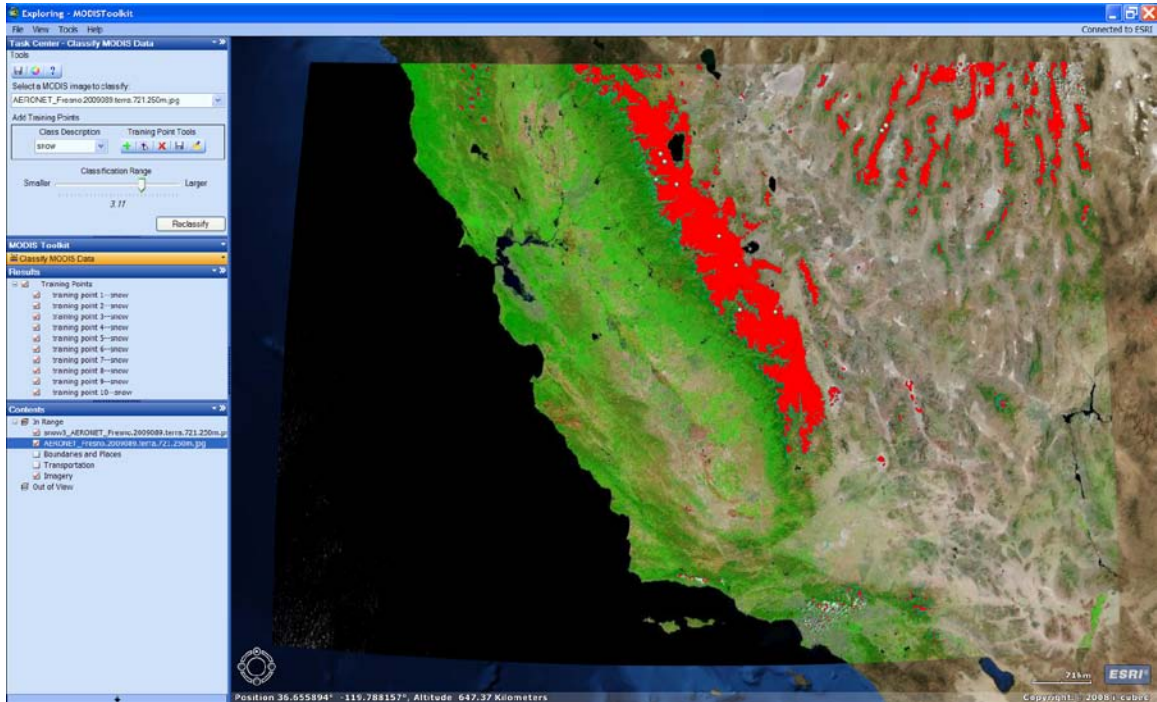
Figure 5-14. Results of image classification performed on a false color MODIS subset to identify pixels representing snow.
