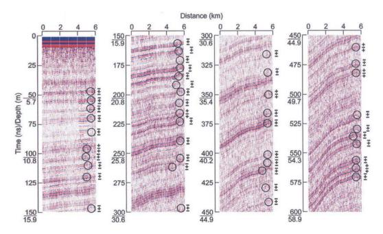
Fig. 4. The top 600 ns of the profile of the first 6 km from core site 00-2. The circled events are wavelets distinguished by peak amplitudes that are at least 3 dB above those of the nearest events.
