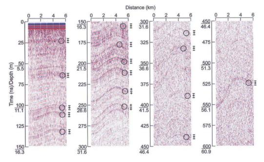
Fig. 7. The top 600 ns of the profile of the last 6 km before the South Pole Station site. The circled events are wavelets distinguished by their amplitudes. The depth scale is based on a density profile from within 100 km of South Pole Station.
