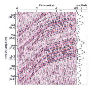
**Fig. 5.** Detail from Figure 4, and a Hilbert magnitude transformation of the trace located beneath the small arrow. The boxed sections highlight horizons with solitary wavelets. The detail shows that some events have the 2.5-cycle structure seen later in the modeling. The amplitude scale of the trace is relative. The energy envelopes of the transform rise as much as 9 dB above the noise level in the troughs.
