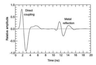
**Fig. 2.** The 400 MHz antenna wavelet form, as revealed by a reflection from a metal sheet buried in firn ( $\varepsilon=1.7$ ). Consequently, the +-+ phase polarity sequence (red-blue-red in the profiles) for the major half-cycles is the inverse of that of the wavelet transmitted into the firn. The direct coupling is through the small air gap between the transmitter and receiver antennas. The bandpass filtering applied to this trace is the same as that applied to all profiles.
