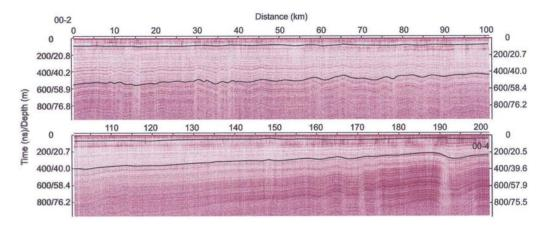
Fig. 3. The top 1000 ns (about 93 m) of the year 2000 profile recorded from core site 00-2 (0 km) to 00-3 (101 km) to 00-4 (202 km). The upper and lower dark lines trace horizons that correspond with 1922 and 1991, respectively. The depth scales at 800 ns are estimates.
