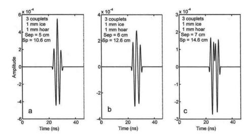
**Fig. 10.** Theoretical reflections from three couplets of ice over hoar, with each couplet separated by 5 cm (a), 6 cm (b) and 7 cm (c). The densities of the hoar and firn are the same as those given in Figure 9. The -+- wavelet structure holds for the three couplets so long as their total span (Sp) does not exceed about 10–11 cm. The peak amplitudes increase with decreasing separation between the couplets.
