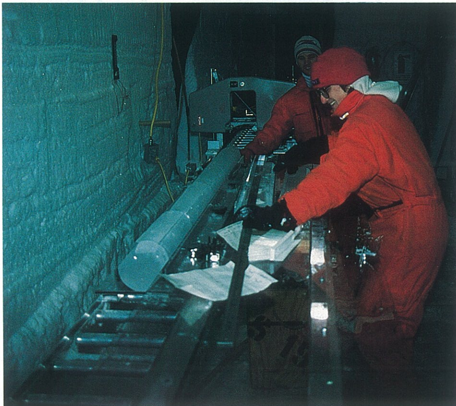
Fig. 4. The horizontal coring station in the core processing line. Courtesy of Michael Morrison, University of New Hampshire.
