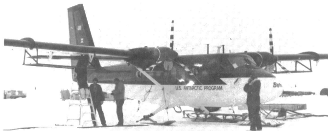
Figure 2. Twin Otter aircraft with antenna mounts for Kansas radar.
