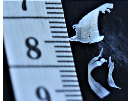
Figure 2.4. Shavings generated with hand plane (<0.05mm thickness)
