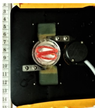
Figure 13.2. Delta T-dish on stage adapter for fish (cm)
