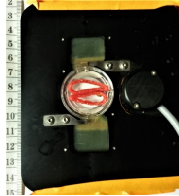
Figure 13.2. Delta T-dish on stage adapter for fish (cm)
