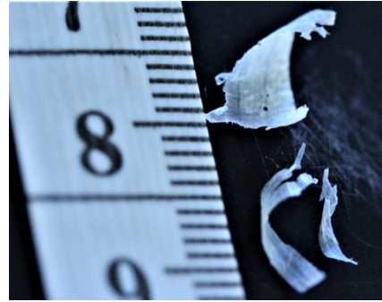
Figure 2.4. Shavings generated with hand plane (<0.05mm thickness)
