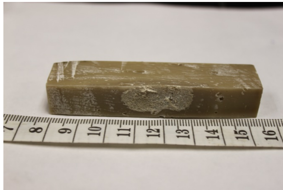
Figure 1.3. View of block after squaring
