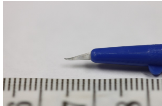
Figure 12.6. 15° Stab microscalpel, slightly bent
