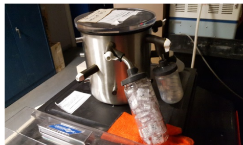
Figure 10: CNF Samples of Varying Porosity with Applied Vacuum on the Freeze Dryer
