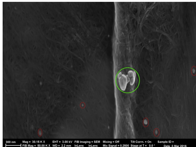
Figure 36: SEM of the Silver Nanoparticles of varying sizes at the surface of a CNF composite matrix
