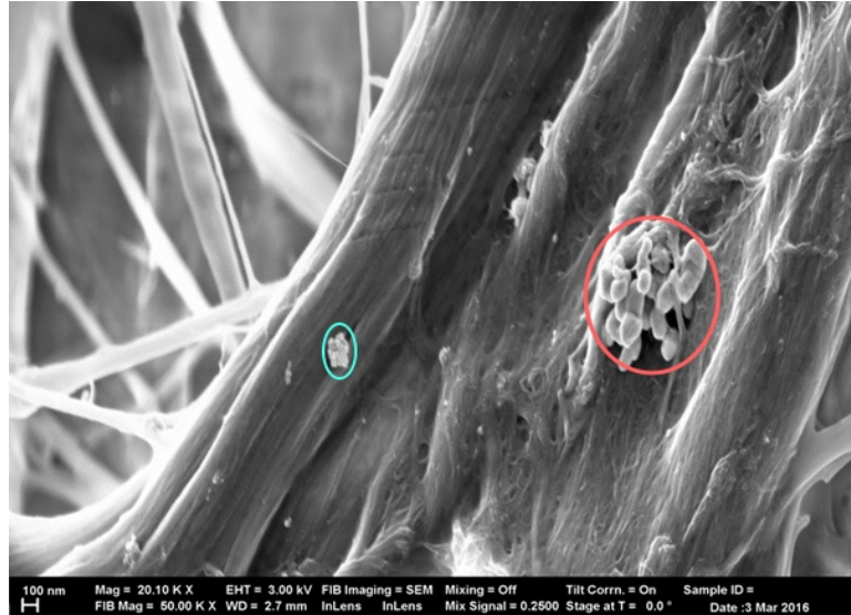
Figure 35: SEM of the Silver Nanoparticles of varying sizes at the surface of a CNF composite matrix
