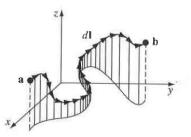
**Figure A.3.** Multiple differential lengths along a curve. The differential lengths here represent infinitely small vectors used to accumulate the effects of a field along a line segment. Image reproduced from E&M course text [58].
