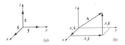
Figure A.1. Cartesian vector notation. (a) Unit vectors for each of the Cartesian axes. Also commonly expressed as *î*, *ĵ*, and *k* for the *x*-, *y*-, and *z*-axes, respectively. (b) A generic vector *A*, or *A*, represented in Cartesian coordinates. Images reproduced from E&M course text [58].
