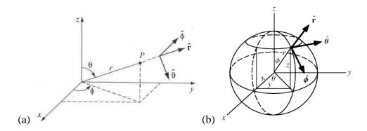
Figure A.5. Notation for spherical coordinates. (a) Standard physics conventions for spherical coordinates. Image reproduced from E&M course text [58]. (b) Standard mathematics conventions for spherical coordinates. Image reproduced from http://mathworld.wolfram.com/SphericalCoordinates.html
