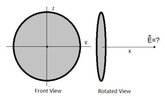
Set up an expression to solve for the electric field a distance, x, far from the center of the sheet.
