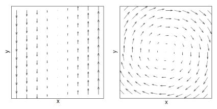
Figure A.2. Two examples of vector fields, showing position dependent vectors. Assuming an origin in the center of the image, the field on the left is expressed by  $\vec{F}(x, y) = x\hat{y}$  and the field on the right is expressed by  $\vec{F}(x, y) = y\hat{x} - x\hat{y}$ . Images reproduced from work by Bollen and colleagues [37].
