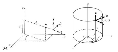
Figure A.8. Notation for cylindrical coordinates. (a) Standard physics conventions for cylindrical coordinates. Image reproduced from E&M course text [58]. (b) Standard mathematics conventions for cylindrical coordinates. Image reproduced from http://mathworld.wolfram.com/CylindricalCoordinates.html
