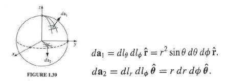
Figure 4.2. Two differential areas in spherical coordinates.  $da_1$  and  $da_2$  depict differential areas for the surface of a sphere and one in the *xy*-plane, respectively. Each is constructed as a product of two differential length components representing changes in each of the angles. Image reproduced from E&M course text [58].
