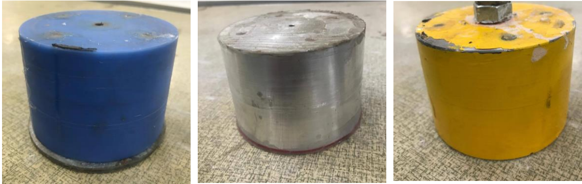
Fig. A.2 Payload model (left: 6.13N, middle: 14.25N, right: 19.95N)
