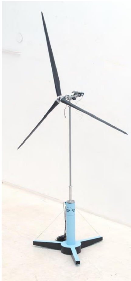
Fig. 3.7 TLP model with wind turbine [5]
