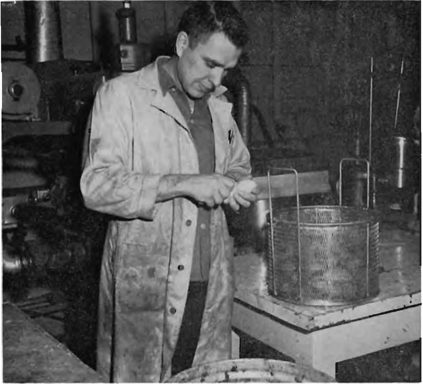
FIGURE 5 Hand trimming after peeling operations
