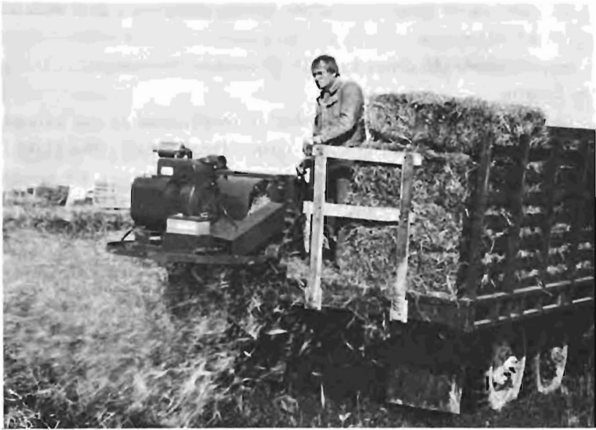
Figure 1. Straw spreading equipment.
