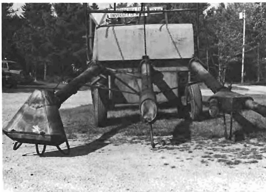
Figure 2. Oil burner with Bosse', Conventional and Economy heads respectively.
