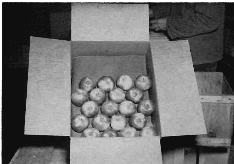
FIGURE 1. Layer packed apples in single wall corrugated box. The packing material is a 3-Ply Cushion and the apples are arranged in an "offset" manner.
