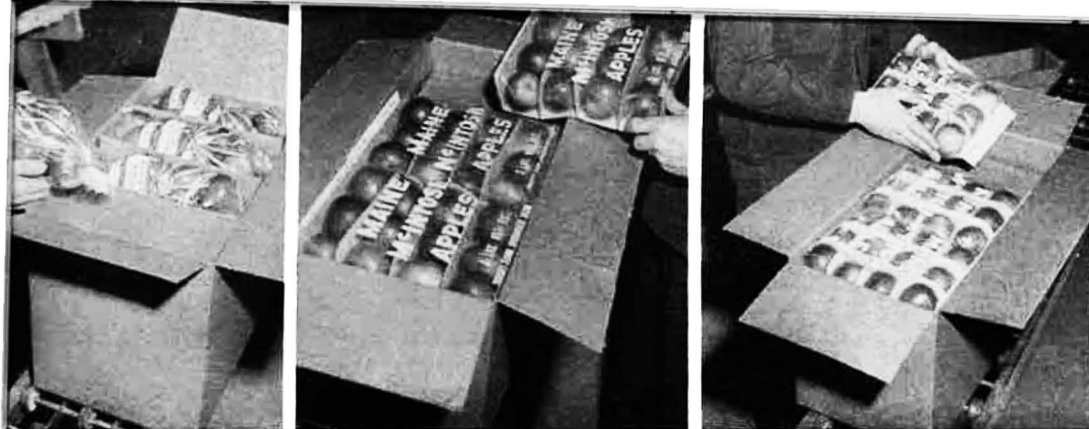
FIGURE 2. Placing consumer packages in master container. At the left the modified jumble-pack poly bag, in the center the poly bag with divider insert and at the right the poly bag with the cell insert.
