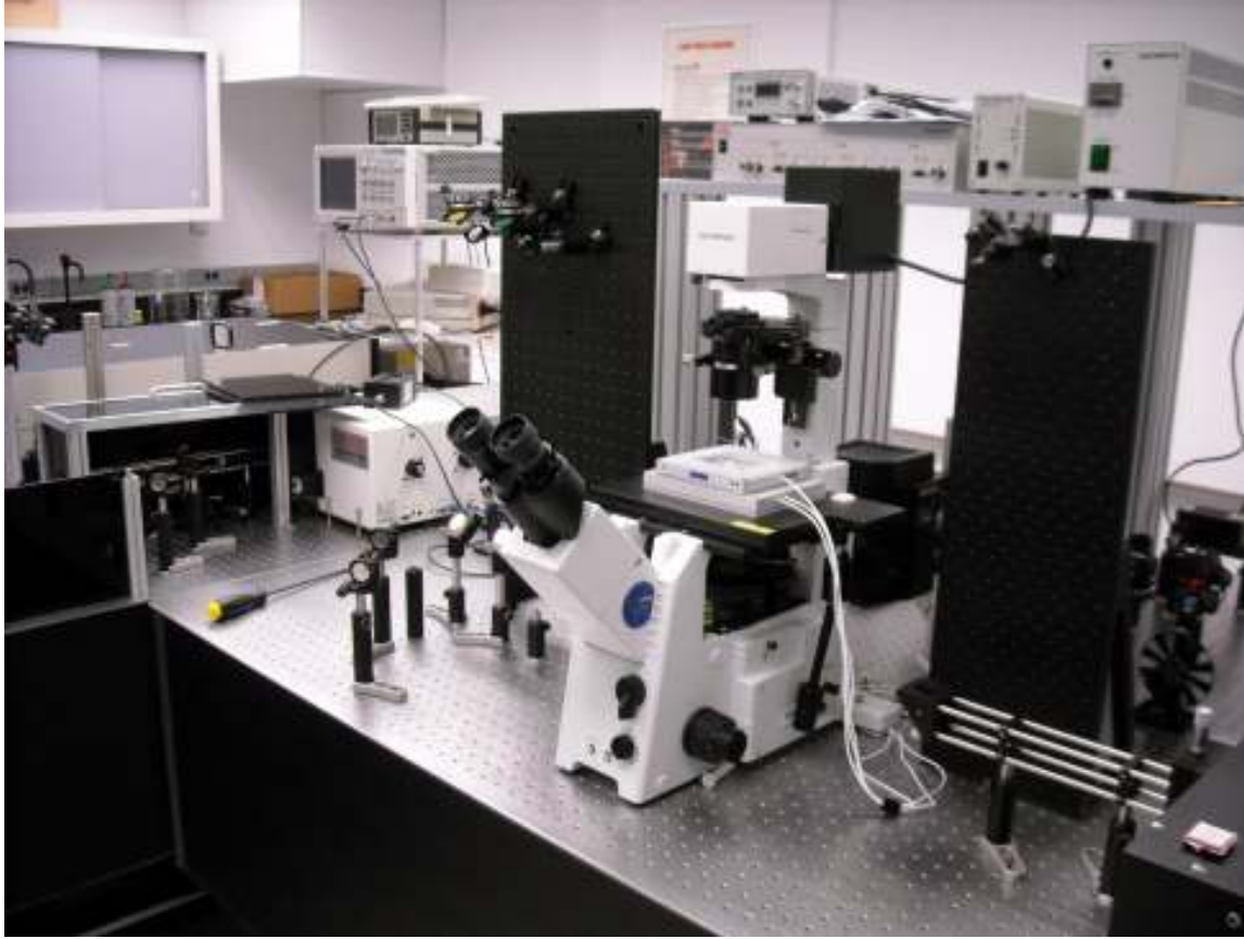
Figure 9. Photo of hybrid SF/FL microscope hardware setup.
