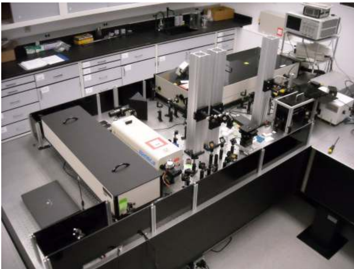
Figure 7. Photo of rebuilt SF spectrometer (FL arm not shown).
