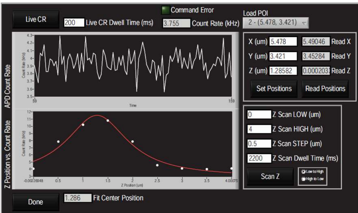
Figure 13. Manual stage positioning, live count rate from the APD, and sample focusing control panel.
