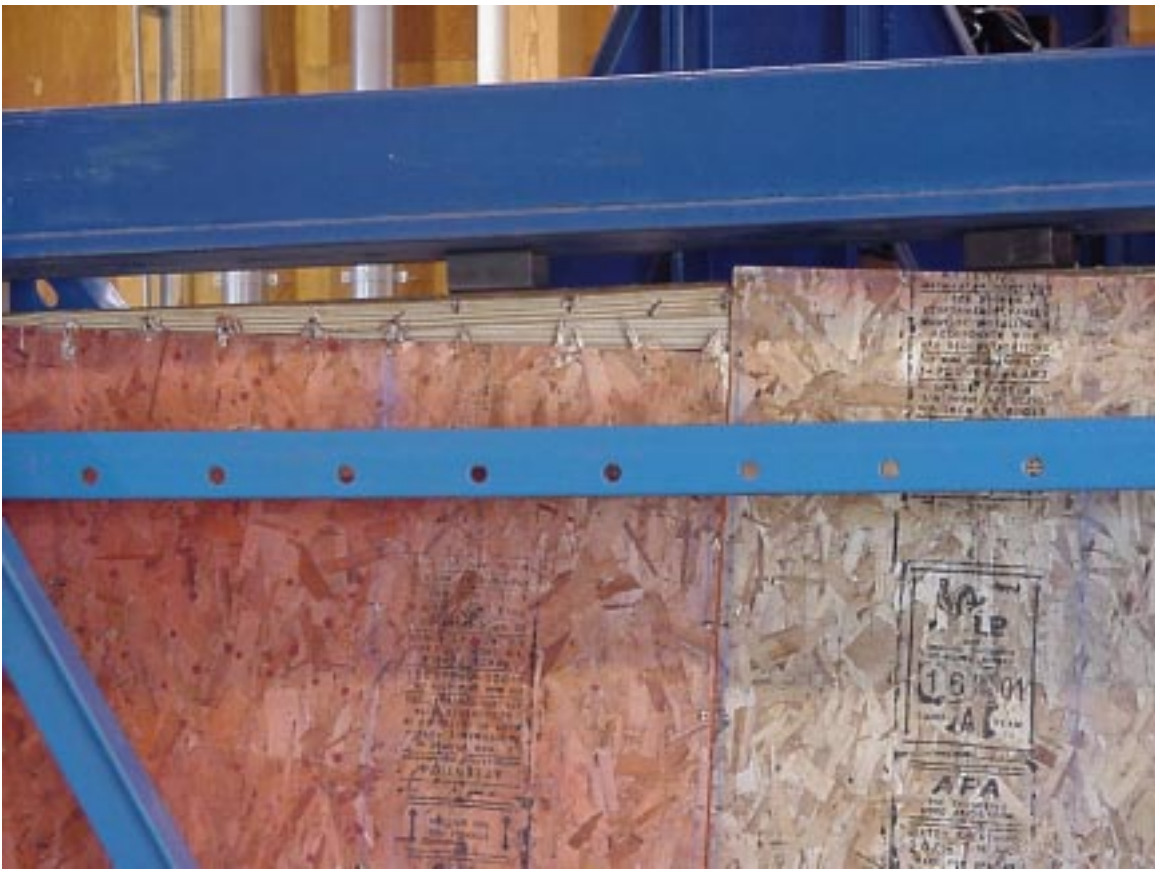
Figure 2: Failed Control Specimen in Shear Wall Test Rig – Note Edge Tear of Nails
