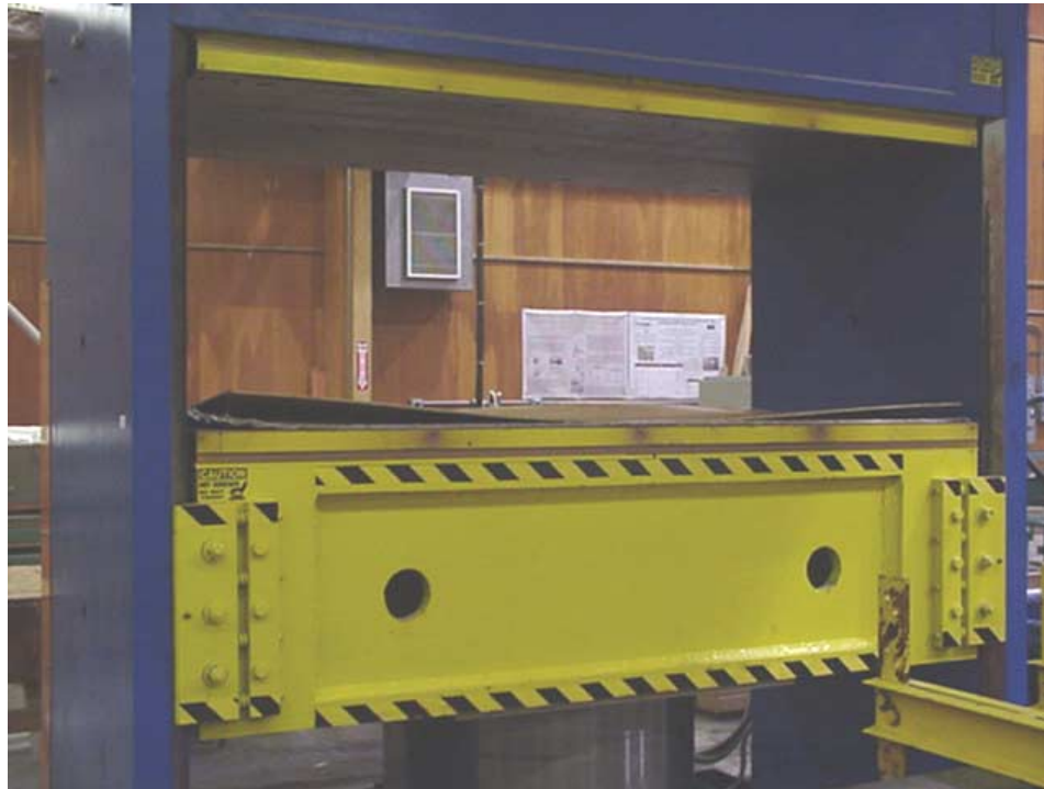
Figure 4.3 Hot Pressing of AOSB Panel.
