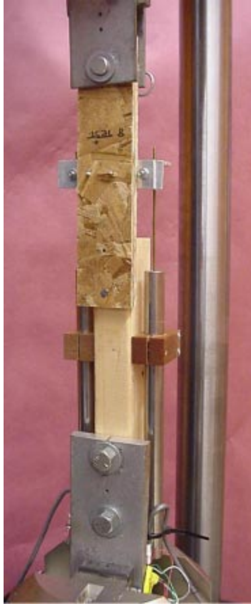
Figure 1: Single Nail Connection Test Set-up
