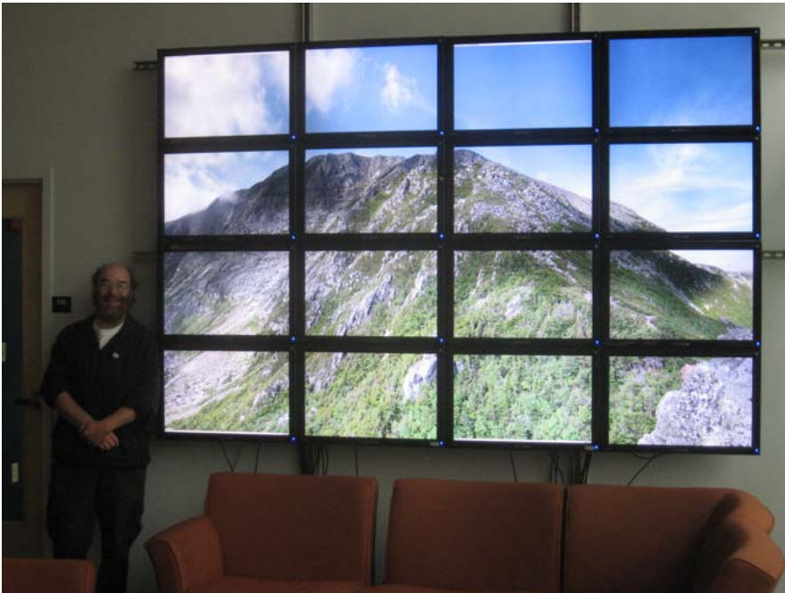
Figure 10: Updated monitors increase the size to 6 ft by 9 ft and resolution to 36 Mpixels.
